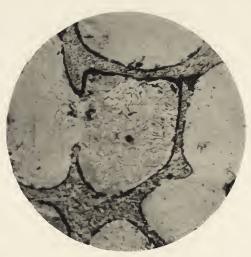
Fig. 23. Iron containing 1.7 per cent. P. and 1.4 per cent C. Magnified 350 diameters.
